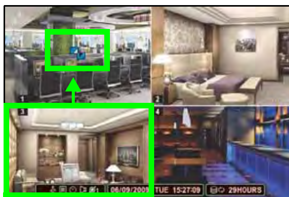
Figure 6.0 Blue Window cursor is in channel 1 Press the 3 button to move channel 3 to the channel 1 position.
