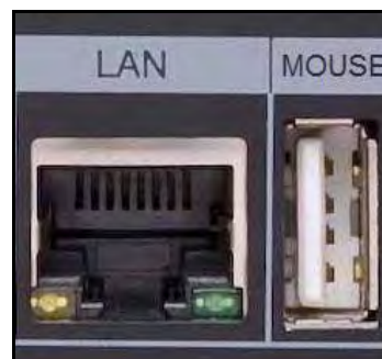
Figure 1.2 Connect an Ethernet cable and mouse
