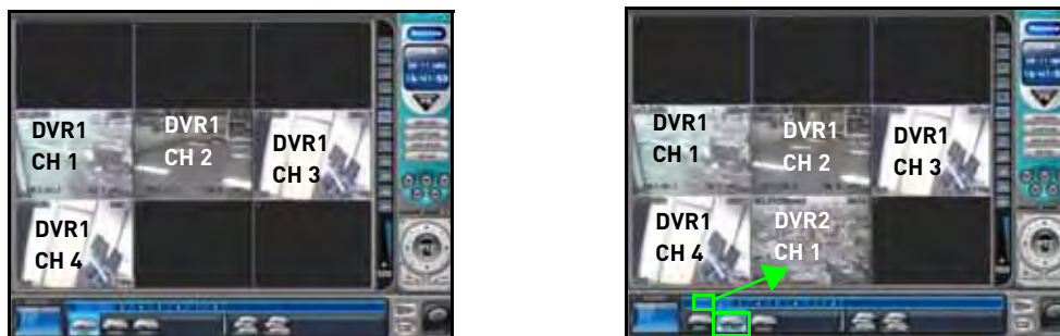
Figure 30.4 Add a Camera—CH 1 from DVR 2 is added to channel 8 on the screen
