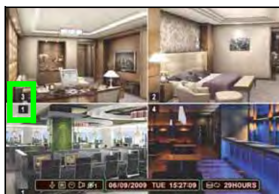
Figure 6.1 Channels repositioned Channel 3 is now in the channel 1 position.
