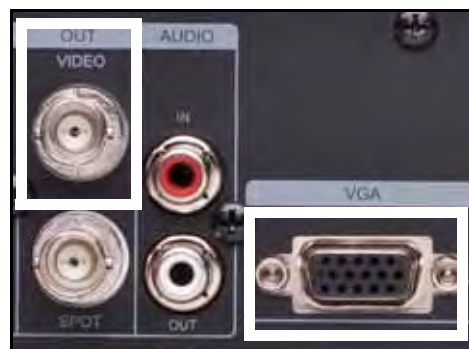
Figure 1.1 Connect to a VGA or CCTV monitor, or a TV
