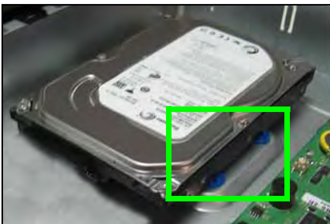
Figure 44.2 Place the HDD on the rubber mounting feet
