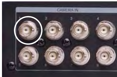
Figure 1.0 Connect BNC cameras to the system
